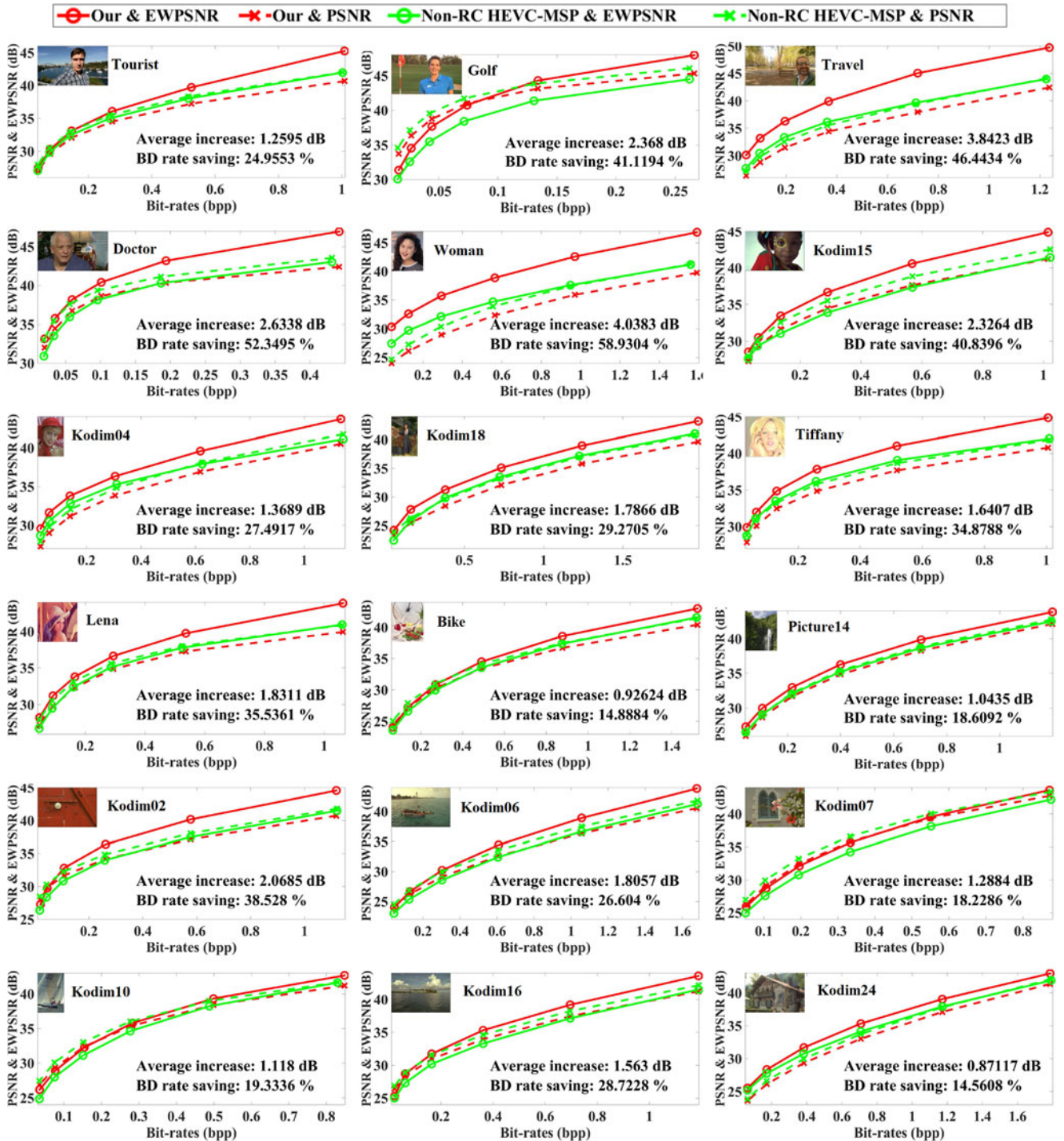
Fig. 4. EWPSNR and PSNR versus bit-rates for our approach and the non-RC HEVC-MSP.
