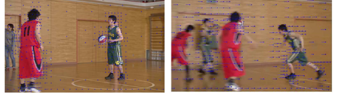
Fig. 6. An example of MV values of all PUs in (a) a frame with no camera motion, and (b) a frame with right-to-left camera motion. Note that the MVs are extracted from HEVC bitstreams. In (a) and (b), the dots stand for the origin of each MV, and the blue lines mean the intensity and angle of each MV. It can be seen that in (a) there is no camera motion, as most MV values are close to zero, whereas the camera motion in (b) is from right to left according to the most MV values.
